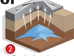
The moisture freezes when temperatures drop, causing the ground to expand and push the pavement up.
