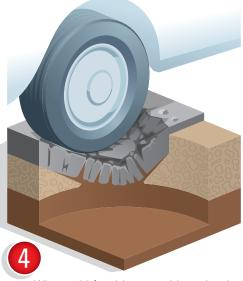
When vehicles drive over this cavity, the pavement surface cracks and falls into the hollow space, leading to the birth of another pothole.
