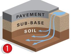
Potholes begin after snow or rain seeps into the soil below the road surface.
